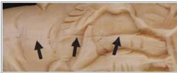
Fig. 5 Mold seams and casting lines Many, but not all, cast resins and plastics show seams. They are often concealed in the pattern as in the piece shown above. Note tool marks at left.
