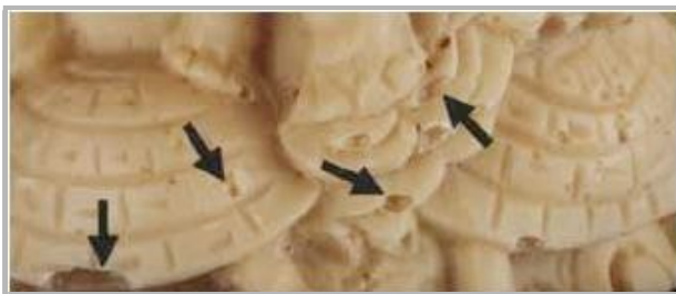
Fig. 2 Broken bubbles in surface of synthetic ivory. Actual size.
