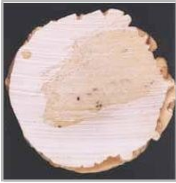
Fig. 8 Be suspicious of rough or obvious tool marks. The deep grooves on this piece appear on the bottom of a supposedly carved tusk. It is a piece of cast resin.
