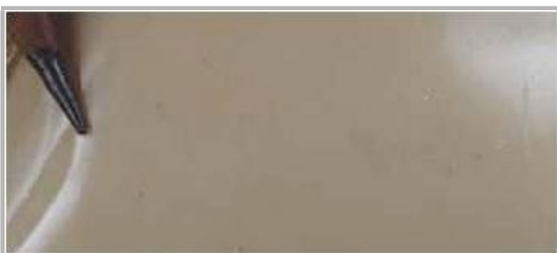
Fig. 3 Surface of synthetic ivory. No trace of grain.
