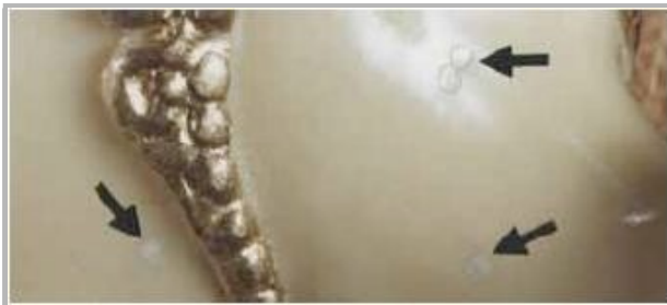
Fig. 1 Pits in surface of synthetic ivory; about twice-actual size
